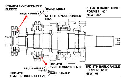
These synchronizers should be used when replacing the 3rd ~ 4th and 5th ~ 6th gear synchronizers in MLS61B transmissions in 1995 ~ 1998 model year vehicles, and in 1999 model year vehicles with Vehicle Identification Numbers prior to the VIN list shown above.
