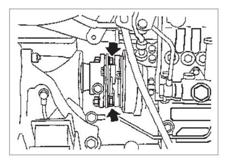
• The <u>correct torque</u> for the injection pump coupler bolt, as indicated on page MA-5-10, should be: **1**: 43 ~ 47 ft·lb (59 ~ 64 N·m) (6.0 ~ 6.5 kg·m).
