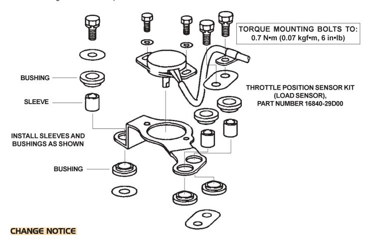
The revised throttle position sensor, kit part number 16840-29D00, includes a mounting bracket with bushings and sleeves as illustrated. Please refer to the recommended torque values for the attaching hardware.
