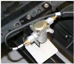
The correct AHI Manifold can be identified by the last 8 digits of the Part Number stamped on the housing
