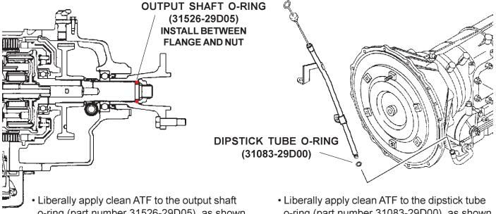
o-ring (part number 31526-29D05), as shown above, before installing.  Liberally apply clean ATF to the dipstick tube o-ring (part number 31083-29D00), as shown above, before installing.
