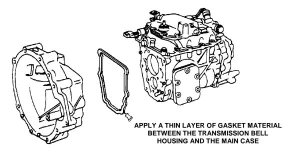
4. Reinstall the transmission bell housing to the main case, the engine flywheel, and the clutch assembly. Uniformly tighten all in a criss-cross pattern to the specifications shown.
