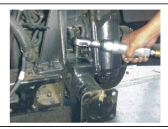
**4.** Using a 19 mm socket, remove the two rear mounting bolts, as shown below, and inspect the bolt threads for damage such as crossed or stripped threads.
