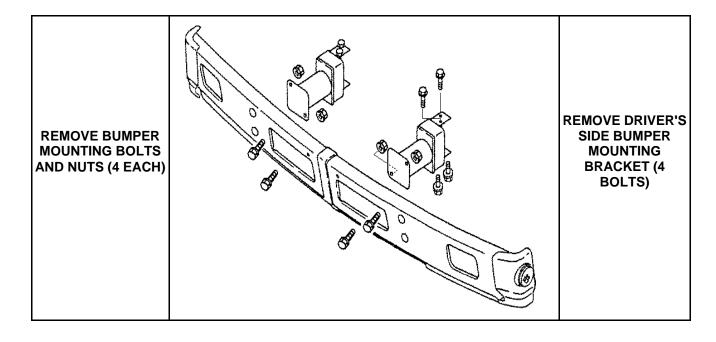
**3.** Using a 14 mm socket, remove the four mounting bolts (two on the top and two on the bottom) from the driver's side bumper mounting bracket as shown below. Remove the bumper mounting bracket from the frame. Save all pieces for reinstallation.
