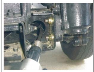
TIGHTEN STEERING GEAR BOX FRONT STUD MOUNTING NUTS
