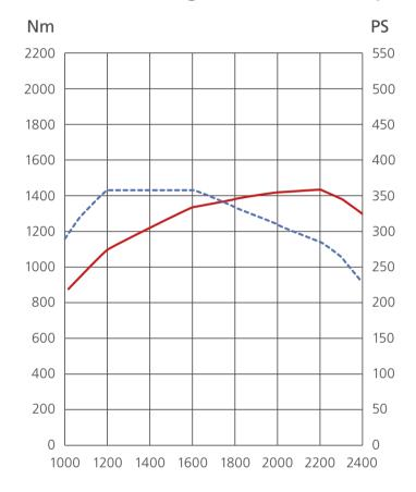
The GH8TA is an in-line six-cylinder diesel engine equipped with a turbocharger and intercooler. The engine produces 357 PS and 1,428 Nm of torque. The engine meets Japan's pPNLT exhaust emissions requirements, which is equivalent to the Euro 6 standards. The engine's functions are controlled electronically. Fuel injection takes place using common rail technology.
