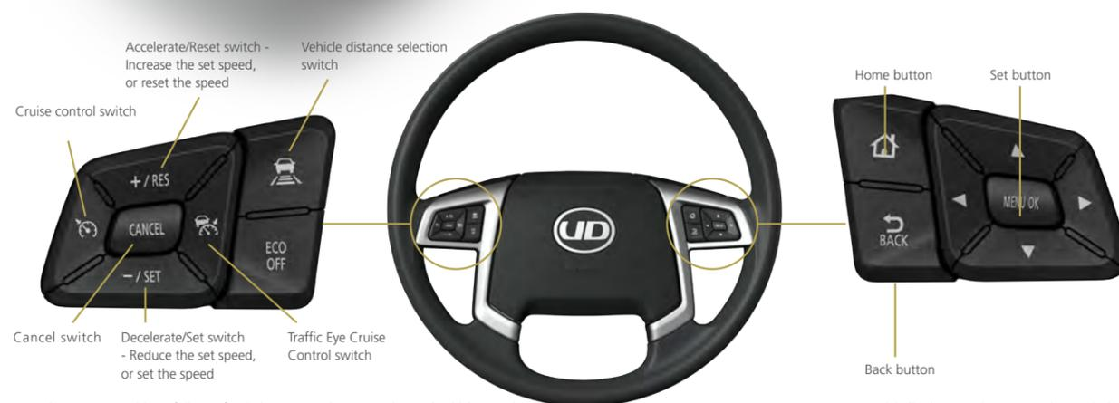
The system provides a full set of switches to set, change, and cancel vehicle speed. There's also an ECO OFF switch to change between ECO mode and ECO OFF mode
