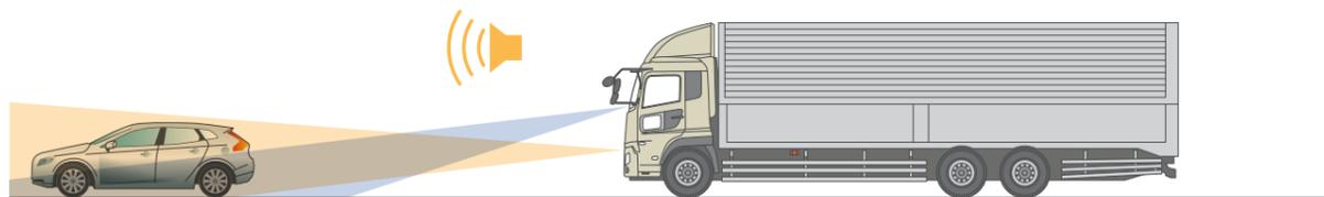
2. While driving, if the system detects a chance of collision with the vehicle ahead, it sounds an alarm and displays a warning indicator to alert the driver.
