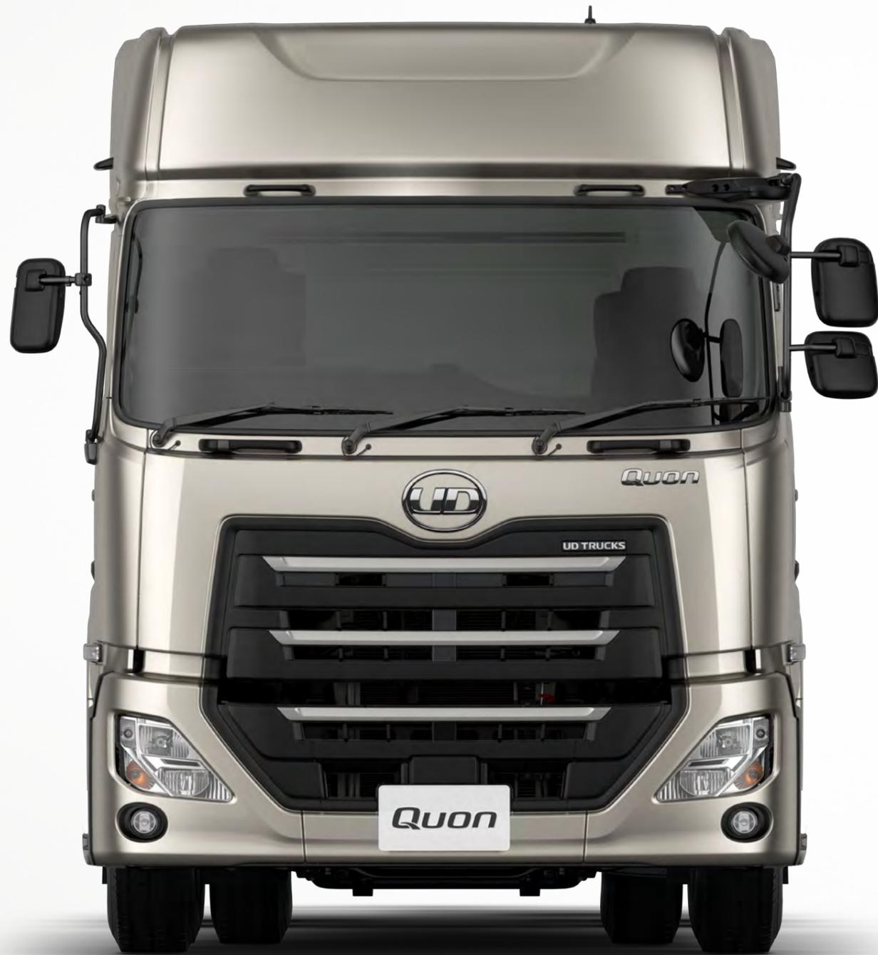
Our design goal was to develop trucks that drivers are proud to drive. As well as a sophisticated functional look, the Quon's aerodynamic shape contributes to fuel efficiency. A low cabin design with two-step entry/exit enables smooth and safe entry to and exit. The headlamps use power-saving, long-lasting LED lamps, for bright, clear light that improves night-time visibility for safer driving.
