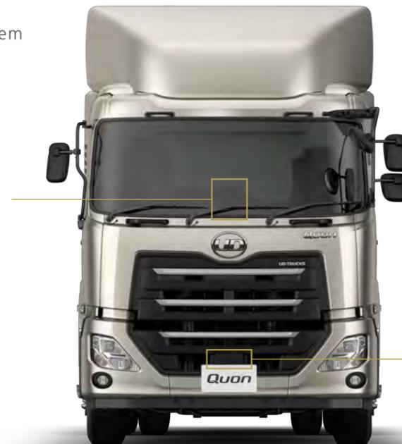
The Millimeter-wave radar functions as the main sensor when detecting the vehicle ahead.
