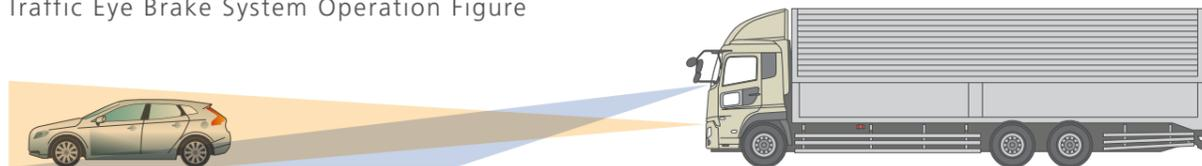
1. Uses both millimeter-wave radar and camera to monitor conditions in front of the truck.
