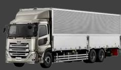
Compared to the conventional full cab, the loading capacity volume has increased by shortening the cab length by 295 mm. The length of the loading platform has been extended to 10.02 meters, allowing extra room for cargo equivalent of two additional T11 pallets, compared to the full cab model.
