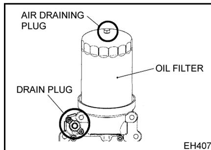
2. The oil will drain within approximately 5 minutes and the cartridge can then be removed.
