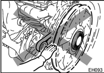
meter". For daily inspections without the sonic tension meter, checking the amount of deflection of the belt using a hand is allowed.
