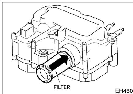
8. Apply a thin film of engine oil to the o-ring on the new equalizing element.
