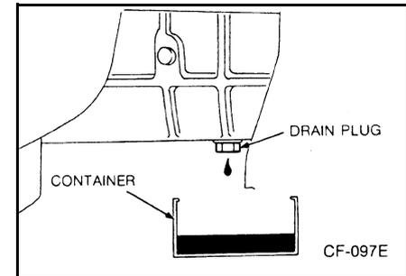
2. After draining, replace the gasket of the drain plug with a new one. Reinsert the plug and tighten the plug.
