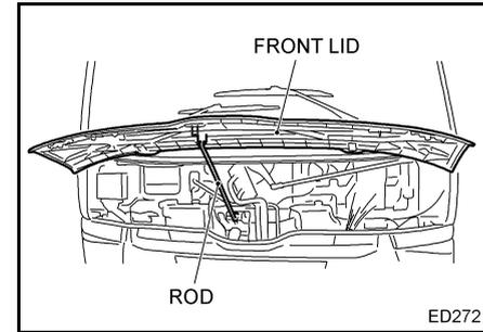
3. When opening the front lid, be sure to set the lever into the hole that is indicated with the mark located on the front lid.
