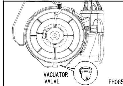
5. Check the rubber seal and hose for breakage and the clamps for looseness. If broken, replace it with a new part. If the clamps are loose, tighten them.
