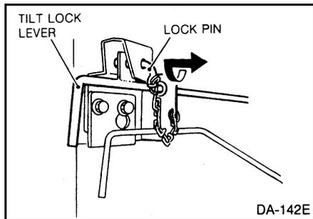
2. Pull the tilt lock lever out all the way. This releases the main hook which holds the cab body to the
