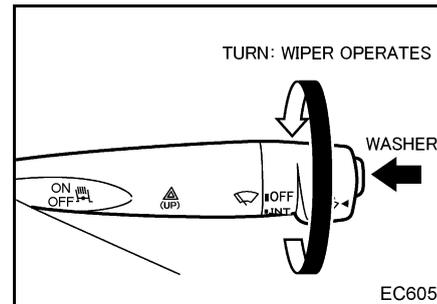
The windshield wiper control is located on the lever mounted on the right side of the steering column.
