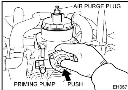
1. Prepare a tray for drained fuel (approx. 2.1 qt [2.0 liter]) and a hose (inner diameter 0.2 in [5 mm], length 3.3 ft [1 m]).
