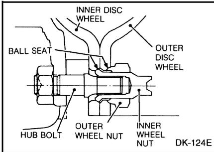
1. Loosen the outer wheel nuts.
