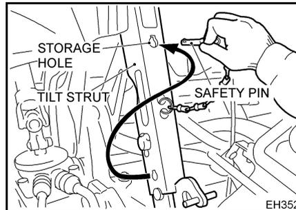
3. While supporting the cab with your hand on the grip, under the left side of the cab, pull the tilt strut rearward and lower the cab.
