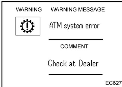
1.The automatic transmission system warnings will be displayed when the TCM detects a malfunction. At this time a diagnostic trouble code (DTC) is set in the TCM and transmission cannot be shifted. Depending on the malfunction, the TCM does not respond to gear shifting operation and the current gear is fixed.
