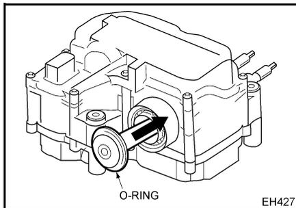
9. Install the filter cover. Tighten the filter cover to the torque specified
