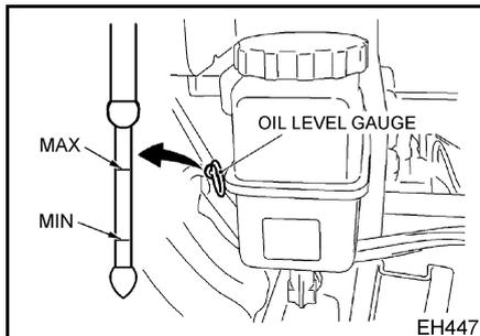
3.If oil level is low, add engine oil of the proper viscosity for the anticipated temperature range during the service interval through the oil filler port located on the valve cover on top of the engine. Do not add oil above the MAX mark on the engine oil level gauge.
