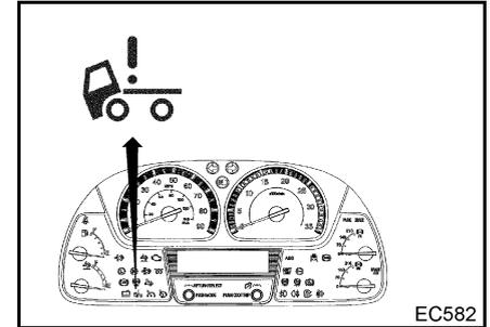
When the warning light comes on and the warning buzzer sounds, immediately move the vehicle to a safe place. To do this, apply the brake slowly.
