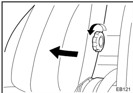
Turn the knob on the outside of the seat toward the front so that the center portion of the seatback will come out slightly to support the lumbar portion of the body. This may be useful in reducing fatigue during long distance driving. The support is adjustable continuously within the adjusting range.
