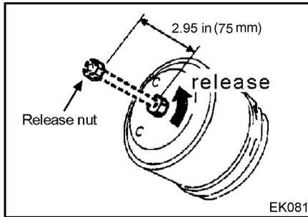
2. Release the release nut by turning it counterclockwise by the specified release amount (Do not use impact wrench).
