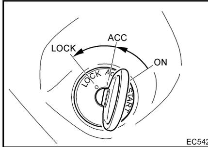
Stop the engine using the ignition key switch. When it is turned from ON to LOCK (OFF), the engine will stop.
