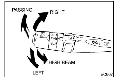
To operate the left turn signal, pull the turn lever on the left side of the steering column down beyond the resistance. To operate the right turn signal, push the lever up beyond the resistance. The lever will automatically return to the neutral position after the turn is completed. When operating the left or right signal, confirm that the TURN SIGNAL AND HAZARD indicator light flashes. When the ON-OFF intervals are unusually short, the bulb is probably burned out.
