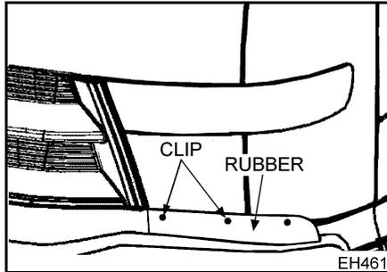
2. Remove the fixing clip from the lower cover, slide the lower cover downward and remove it.
