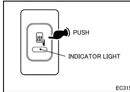
This switch is located at the right side of the steering column.
