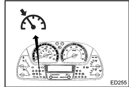
3. When the preferred speed is reached, press and release the Cruise Control Set and Coast Button located at the end of the combination switch.
