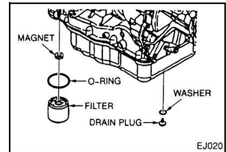
2. Remove the drain plug from the oil pan and allow the fluid to drain into a suitable container.
