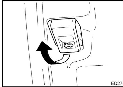
2. Disengage the front lid hook. Push up the front lid and secure it with the rod.
