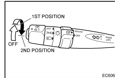
Turn the knob on the end of the switch lever to the 1st or 2nd position to operate the following lights.
