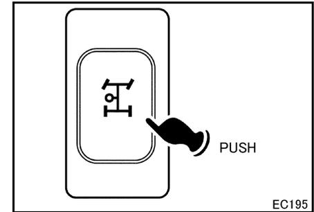
This switch located on the instrument panel to the left of the steering column, couples and uncouples power flow to the transmission PTO. To turn the PTO ON, idle the engine, depress the clutch pedal fully, and depress the switch. The PTO indicator and operation message will come on. To turn the PTO OFF, idle the engine, depress the clutch pedal fully, and depress the switch. The PTO indicator and operation message will go out.
