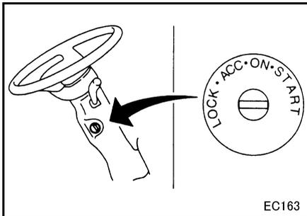
The ignition key switch, located on the right side of the steering column, has four positions:
