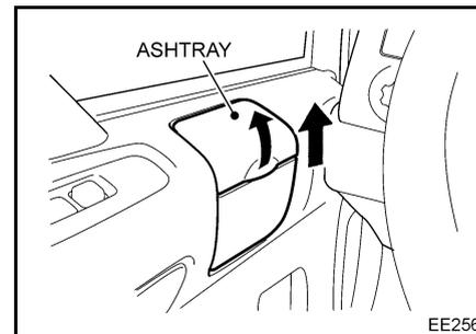
The ashtray is located inside of the right and left doors. To open the ashtray, pull the tab upward. To remove the ashtray for cleaning, pull the tray upward.
