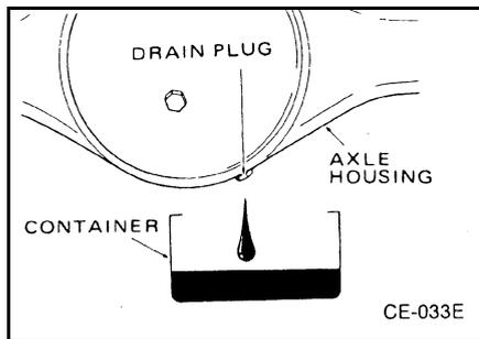
2. After draining, replace the gasket of the drain plug with a new one. Install the plug and tighten the plug.
