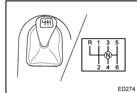
The transmission gear shift lever is located on the right of the driver's seat. When shifting gears, depress the clutch pedal fully and move the lever firmly. When the shift lever is moved into reverse, the backup lights come on and the backup buzzer sounds. The backup lights and buzzer are located on the rear of the vehicle.
