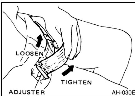
To tighten the seat belt, pull the loose end toward the belt anchorage until it fits snugly.
