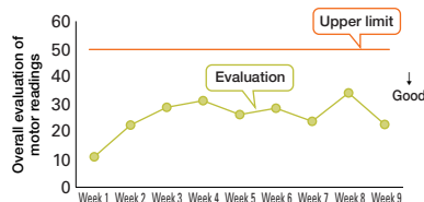
Spray pump motor standard monitoring values
